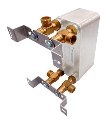
The mounting bracket is available in three variations, depending on the size of the connections (DN20, DN25, and DN32). The threaded components (excluding screws) are made of MS58 brass, while the mounting rails are made of stainless steel.
